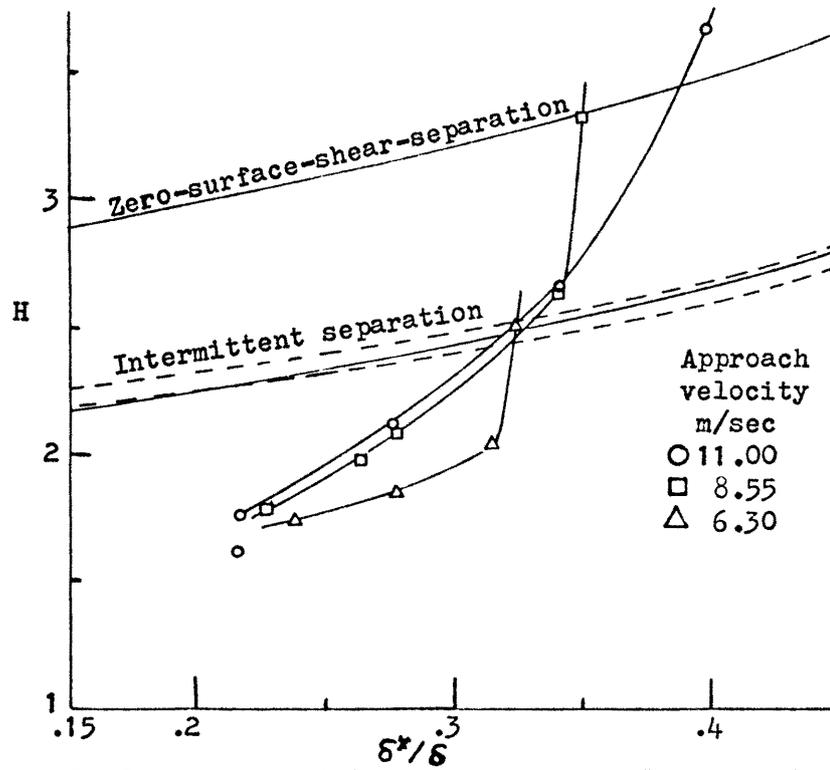
Figure A-7. Comparison of the velocity profile parameters with the Sandborn-Kline separation correlations.
