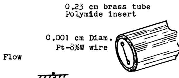
Figure 3. Surface hot wire-heat transfer sensor.
