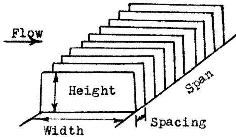
0.014 cm thick aluminum sheet used for construction. Each fin is made with a 90 degree bend at bottom of the width of the spacing. Each fin is glued to a 0.014 cm thick sheet. The sheet is in turn glued to the wind tunnel surface.
