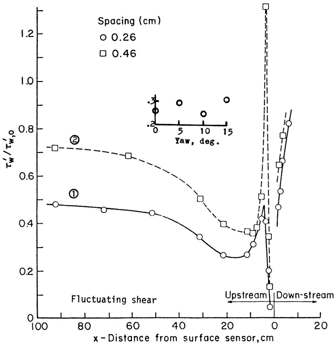
Figure 5.- Variation of the mean and fluctuating surface shear for two sets of fins.
