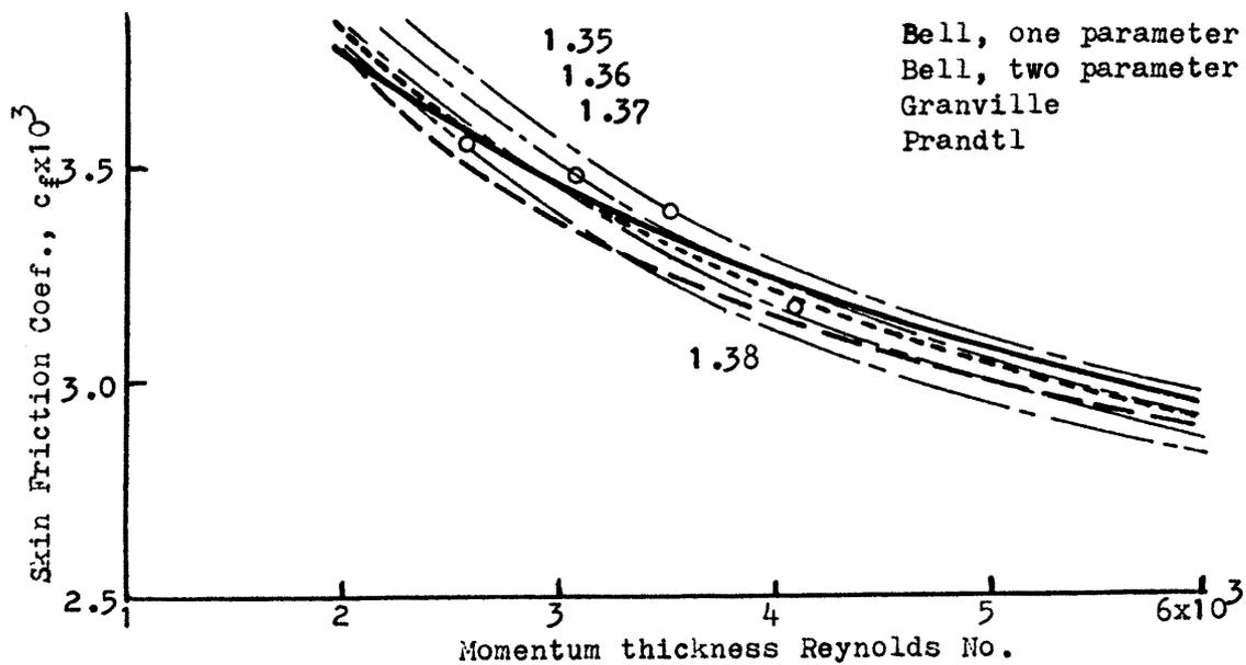
Figure 4.- Local shear stress determination.
