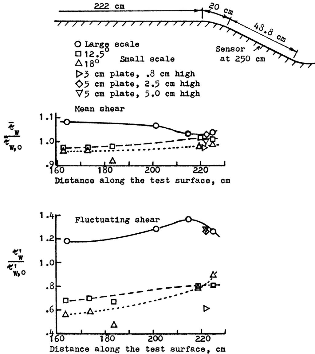
Figure 11.- Effect of vortex generators and deflection plates on the surface shear in adverse pressure gradients.
